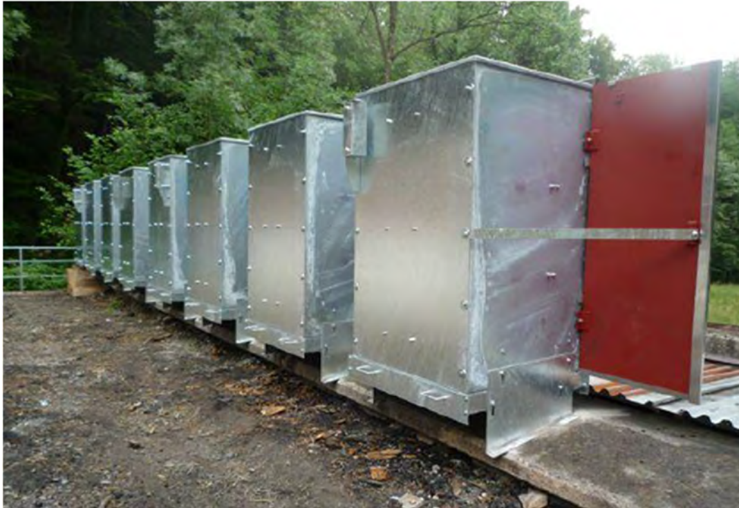
Figure 23 Back of the bullet trap cassettes lined with steel plates. Leu + Helfenstein AG (Switzerland)
