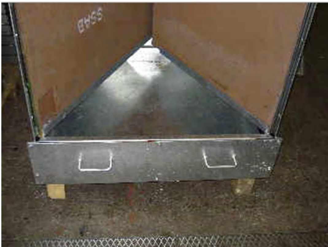
Figure 24 Interior of a bullet trap cassette lined with steel plates. Leu + Helfenstein AG (Switzerland)
