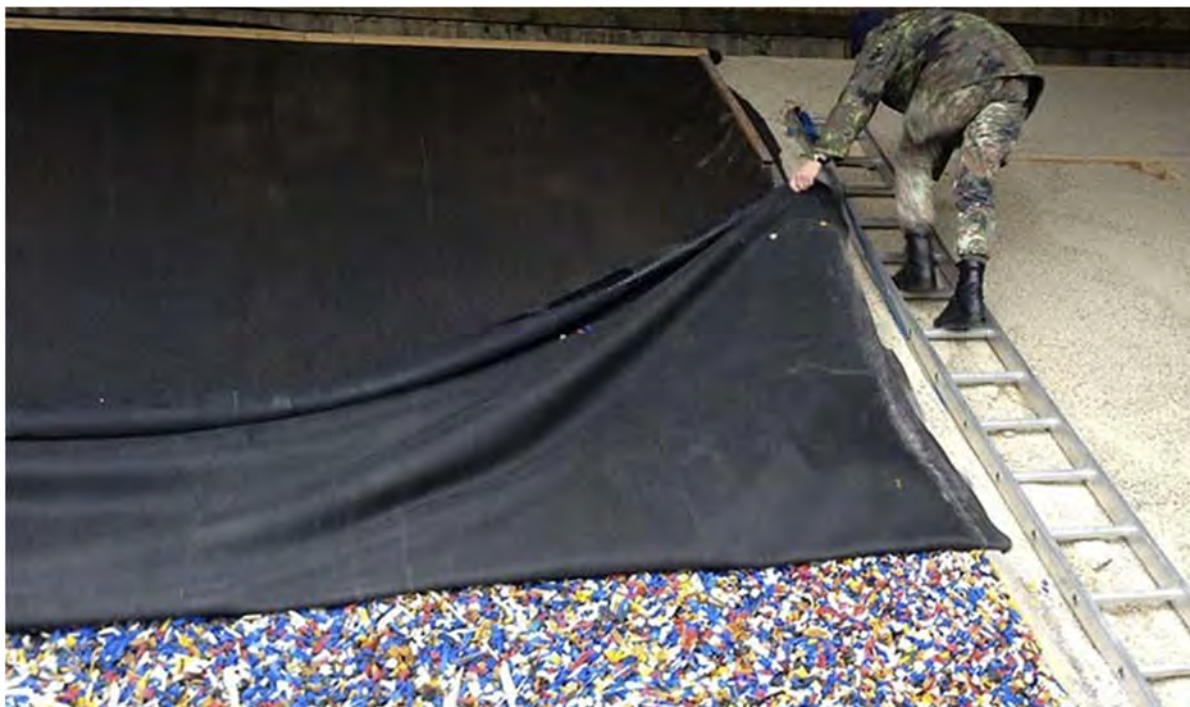
Figure 12 Granulated plastic bullet trap with a cover. Excerpted from https://www.obsima.no/produkter/skyte-og-ovingsanlegg/rikosjettsikring/sgp-rutec-r5000-granulat
